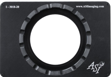
Warner Stage Heater Insert (Series 20 and 30) (I-3018-20 or I-3018-30) The I-3018-20 insert provides a 91.4 mm (3.60") diameter by 9.1 mm (0.35") deep opening to hold a Warner stage heater, plus offers 360 degree continuous rotation. This is for the Series 20 Warner Incubator. The I-3018-30 insert provides a 91.4 mm (3.60") diameter by 9.1 mm (0.35") deep opening to hold a Warner stage heater, plus offers 360 degree continuous rotation. This is for the Series 30 Warner Incubator. Depth from top of Insert: 9.1 mm Overall Thickness: 10.0 mm
