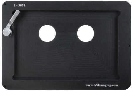
Mouse-Holding Insert (I-3024) The I-3024 insert provides a 128.0 mm by 86.1 mm (5.04" x 3.39") lowered platform for in vivo mouse imaging. (This is the same opening size that accepts an SBS Standard multiwell microplate.) There are two 21.0 mm (0.83") off-axis holes for viewing from below. The unit's recession places the bottom of the specimen about 8.5 mm below the top of the insert. Depth from top of Insert: 8.5 mm Overall Thickness: 9.5 mm
