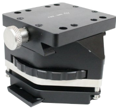
XY Precision Centering Stage Commonly used to center devices over microscope objective; 25 mm X travel, 8 mm Y travel, load capacity 25 kg, resolution~ 10 microns CDZ-1000
