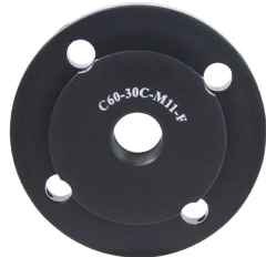
C60-30C-M11-F C60 38 mm ring to 30 mm cage rods adapter. It has provision for 10 mm or 12.5 mm glue-in lens, and 56 mm O.D. x 9.4 mm I.D. In addition, it comes with M11 female threads for collimator.
