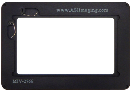
PARC High-Rise 96-Well Slide Insert (I-3028-B96) The I-3028-B96 insert provides a 128.3 mm by 86.1 mm (5.05" x 3.39") opening to hold a PARC 96-well slide. (This is the same size opening that accepts an SBS Standard multiwell microplate.) The unit is recessed to place the bottom of the slide about 1.5 mm below the top of the insert. NOTE: This insert is the equivalent of a High-Rise version of the I-3020. Depth from top of Insert: 1.5 mm Overall Thickness: 8.0 mm
