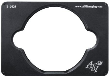
Semiconductor Wafer Insert (I-3025) The I-3025 insert provides a 100.1 mm (3.94") partially circular opening to hold a standard 100 mm semiconductor wafer. The unit is recessed to place the bottom of the wafer about 7.5 mm below the top of the insert. Depth from top of Insert: 7.5 mm Overall Thickness: 8.0 mm
