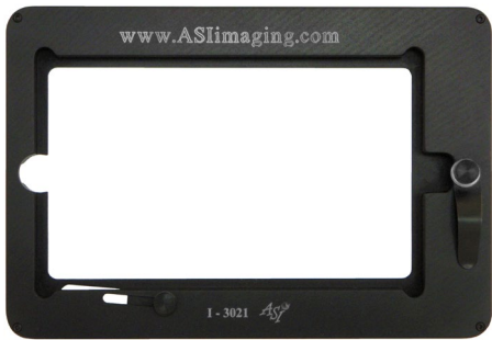
PARC 3x5 Slide Insert (I-3021) The I-3021 insert provides a 127.5 mm by 76.7 mm (5.02" x 3.02") opening to hold a PARC 3x5 slide. The unit is recessed to place the bottom of the slide about 7.2 mm below the top of the insert. Depth from top of Insert: 7.2 mm Overall Thickness: 8.0 mm
