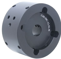
C60-30C-12.5 LM C60 38 mm ring to 30 mm cage rods adapter with female ring mounts. It can be used without cage if needed it. Provision for 12.5 mm lens held by set screws (e.g. cylindrical lens).
