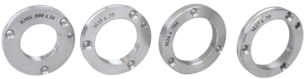
Objective Adapters C60-OBJ-M25 - Objective adapter for Nikon M25-0.75 threads (NIKON CFI 60 series objectives). C60-OBJ-RMS - Objective adapter for RMS threaded objectives (Olympus). C60-OBJ-M26 - Objective adapter for M26 x 32 TPI threads (Mitutoyo). C60-OBJ-M27 - Objective adapter for M27 x 1.0 (Zeiss).
