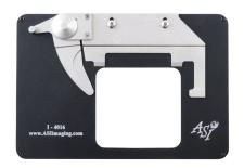
**Slide Insert with Finger Flush Version (I-4016)**This is a special version of the I-4012 that places the bottom of a slide flush with the top of the insert. The insert has a milled-out bottom to allow objective clearance. Available for upright microscopes that cannot move close enough to achieve correct focusing, however, Kohler illumination may not be possible with this insert.
