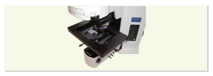
The PZMU-2000 is a precise piezo Z-axis stage that can be attached to the top of a microscope's existing XY stage or be used in stand-alone applications. On select models of microscopes, ASI can mount a PZMU-2000 to an OEM stage. We can procure a manual OEM stage for you if necessary.
