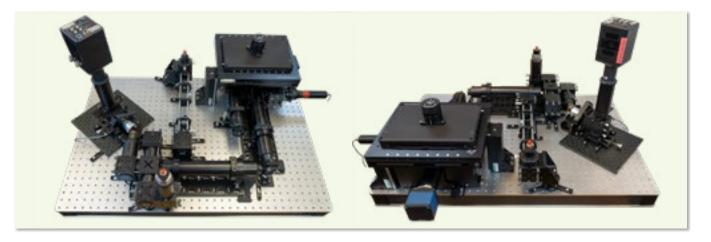
The single-objective light sheet geometry – known in the literature as OPM, SCAPE, SOPi, eSPIM, and SOLS – enables 4D fluorescence imaging of biological samples at high speed and low light dose with conventional sample mounting. Previously such a microscope had to be homebuilt; now ASI is making this transformative technology broadly available in collaboration with Leica Microsystems.
