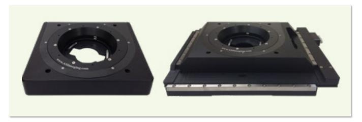
The PRS-1000 Precision Rotary Stage utilizes ASI's proven precise control through the use of closed-loop DC servo motors and angle encoded out drive. The low profile design with the ability to be integrated into our MS-2000 XY stages offers flexible usage. Standard versions have a Ø 95 mm clear through aperture, use all of ASI's C size inserts, and have M3 tapped holes on 125 mm D.B.C. The PRS-1000 is also available with solid top plates for vacuum applications and M6 on 25 mm centers.
