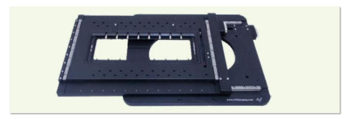
The MS-2500-Ti XY low-profile stage has been designed to provide 100 mm (4") of Y-axis travel with an extended 250 mm (10") of X-axis travel. This extended travel makes for easy robotic loading or for holding more samples per stage insert. The MS-2500 stage accepts either standard 160×110 or wide 283×110 stage inserts. Total stage thickness is only 54.1 mm (2.13"), and only 29.3 mm (1.16") from its flat obstruction-free top to its bottom mounting surface.
