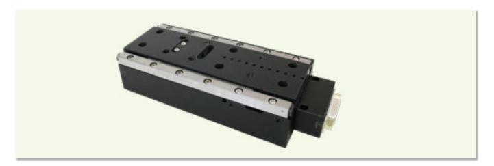
LS linear stages provide sub-micron accuracy, deriving their precise control by using closed-loop DC servo motors and employing high-resolution rotary encoders for positioning feedback. An optional linear encoder can be added to the unit to provide even greater positioning accuracy.
