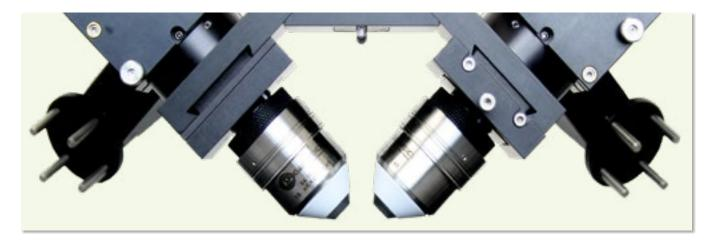
ASI and Special Optics have developed three objective lenses designed for light sheet microscopy of cleared tissue samples, including ASI's ct-dSPIM. These objectives work in any refractive index media without a correction collar because of a unique curved first surface. They are robust to immersion in harsh media including DBE and BABB. The large working distance enables imaging samples that were previously inaccessible.
