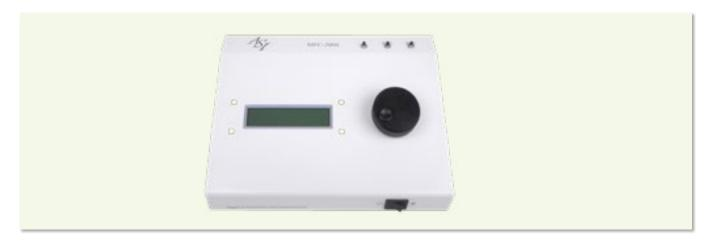
The MFC-2000 has been designed to provide a high resolution and highly repeatable, means of controlling the focus/Z-position of the microscope stage. Precise control of the microscope's focus is obtained through the use of a closed-loop DC servo motor employing high resolution encoders for positioning feedback. By using closed-loop control of the focus position, there is no chance that the focus point can be lost as can occur with open-loop stepper motors.
