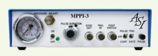
The Milli-Pulse Pressure Injector, MPPI-3 produces gas pressure pulses to an injection pipette. The unit offers precise linear control of both pressure and pulse duration. Alternatively, an external source such as a signal generator can be used to control the pulse width and rate.
