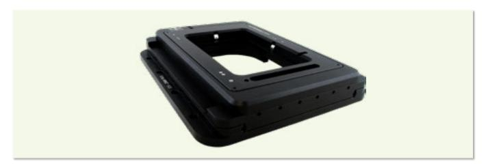
The US-2000 has been designed to provide an ultra-stable, high resolution stage for super resolution microscopy, especially localization microscopy. Materials were selected to minimize thermal drift not only in the X- and Y-axes, but Z-as well. It utilizes crossed-roller bearings, a high precision lead screw, and closed-loop DC servo motors. Though the US-2000 is the most thermally stable of ASI's stages (without feedback), other stages offer longer travel and even better repeatability.
