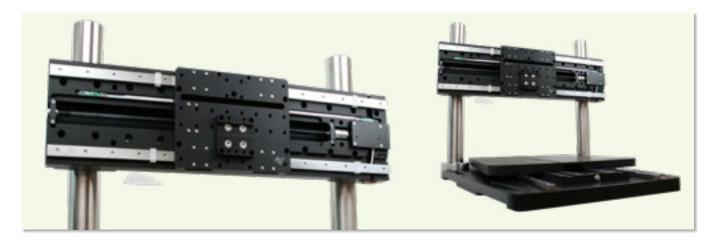
GTS-Series Gantry Translation Stages offer three precision closed-loop DC servo motor linear actuators available in a range of travels. The standard 15-inch unit, shown, allows 380 mm (15") of travel in the X- and Y-coordinates and 100 mm (4") of travel in the Z-axis, with smaller and larger travel ranges available. An optional fourth axis controls the zooming video microscope, shown, available with zoom ranges as high as 16X.
