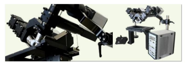
The ct-dSPIM is a flexible and easy-to-use implementation of Selective Plane Illumination Microscopy (SPIM) that allows for dual views (d) of large samples such as cleared tissue (ct).
